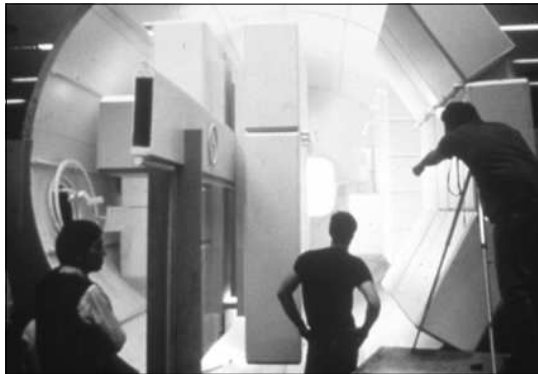
Figure 4 A full-scale mockup of a hybrid Space Station Laboratory and Habitation Module: Support Rails around Enclosure periphery; Utility Beam through center; Disc Connector on Utility Beam, Transpacs (transportable storage) mounted to rails and beam; Special Function Device (camera mount) on Enclosure wall.
