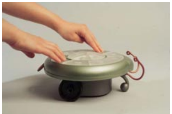
Figure 4 MusiCleaner: a mobile mini vacuume cleaner controlled bu music input
